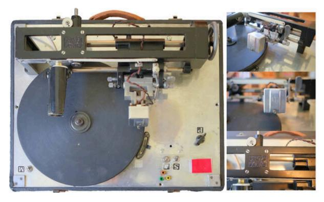
(Trans)portable 78 rpm recorder based on a **Carobronze Dual** turntable and a **Pierre Clément** cutting head. The lathe allowing the radial movement of the arm comes from **Poltz Frères** in Paris. Our equipment has been somewhat customize... there is normally the possibility of a second control arm.
