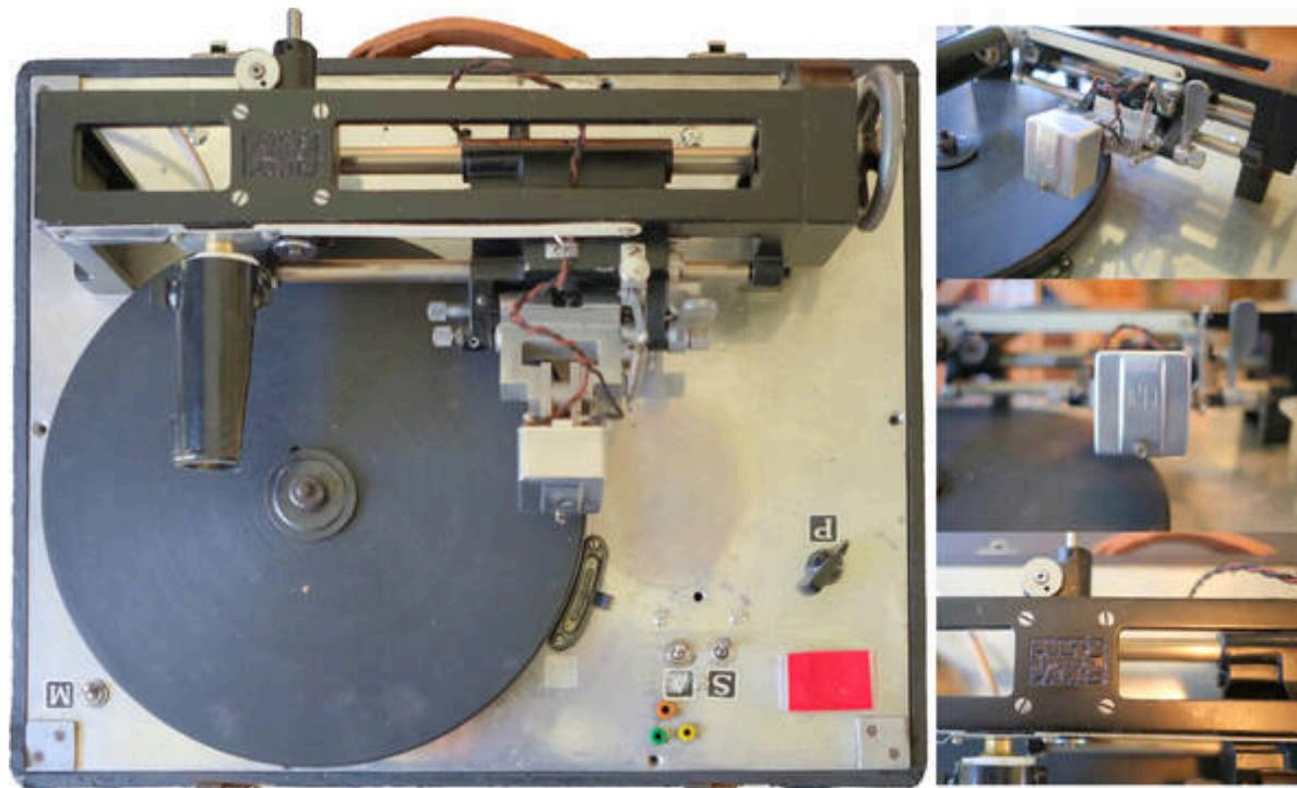
(Trans)portable 78 rpm recorder based on a **Carobronze Dual** turntable and a **Pierre Clément** cutting head. The lathe allowing the radial movement of the arm comes from **Poltz Frères** in Paris. Our equipment has been somewhat customized... there is normally the possibility of a second control arm.
