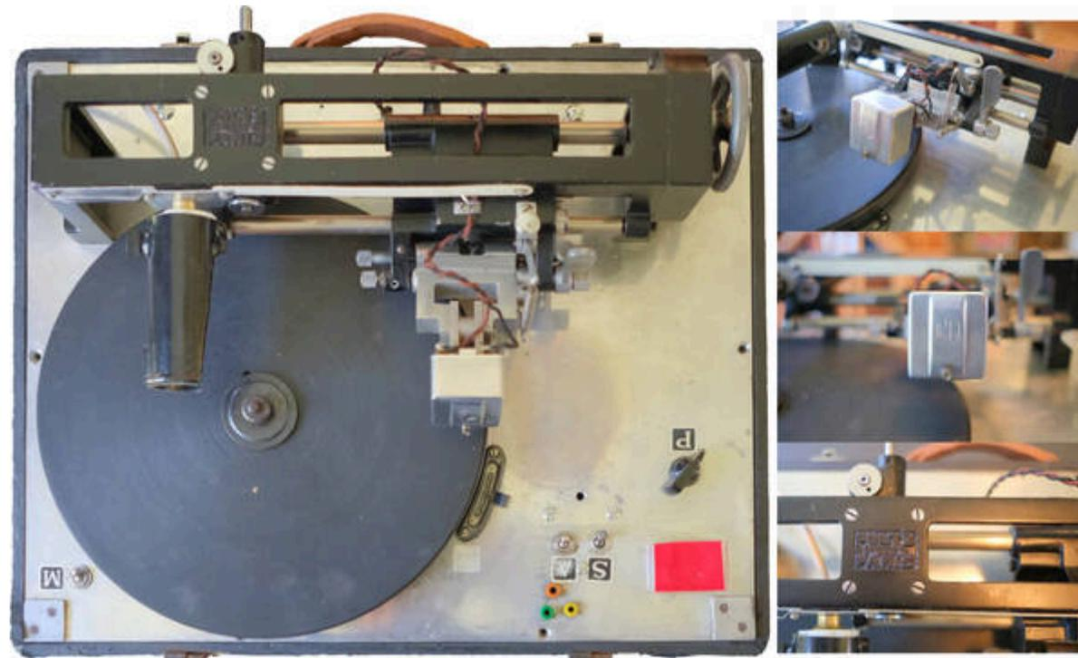
(Trans)portable 78 rpm recorder based on a **Carobronze Dual** turntable and a **Pierre Clément** cutting head. The lathe allowing the radial movement of the arm comes from **Poltz Frères** in Paris. Our equipment has been somewhat customize... there is normally the possibility of a second control arm.
